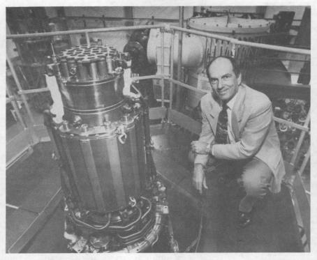
SCOPING OUT TOPAZ — Dan Hartley, VP-6000 and Manager of the Energy and Environment Sector, is seen here with a TOPAZ Russian space nuclear power system. Two of the reactors installed for research purposes near the University of New Mexico (UNM) are being studied by a team of scientists from Sandia, UNM, Los Alamos National Lab, and Phillips Lab, and several Russian scientists.
